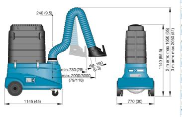
FilterCart Original mobile filter unit for light welding and extraction applications. FilterCart Original includes Extraction Arm Original with an integrated spotlight, which optimizes the user-friendly design. If a larger working range is needed, the 3 m (10 ft.) long arm version is recommended.
